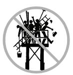
Occupants, equipment and materials shall not exceed the maximum platform capacity.
