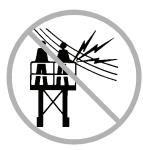
Keep away from the machine if it contacts energized power lines or becomes electrically charged. Personnel on the ground or in the platform must not touch or operate the machine until the energized power lines are shut off.
